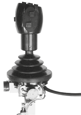
With a linear-motion potentiometer for Z axis and special knob with 7 push-button switches. ▪ S90JAM-ZZ-36R3G
